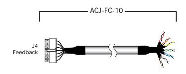
This cable plugs into drive J4 and consists of seven twisted-pairs of AWG 24 wire. Each pair has a black and colored conductor. The chart above shows twisted-pairs in the rows. E.g. one pair goes to pins 1&8, another pair to pins 2&9, etc. Cable termination is flying leads for connection to customer motor feedback encoder.
