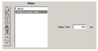
■ Enter the value directly or enter the number (R0-R31) of an Indexer 2 Program register. See Using Registers to Pass Values to Functions (p. 33).
