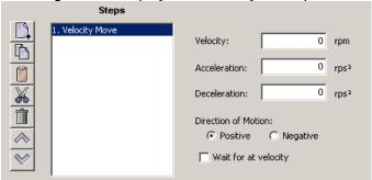
Choose appropriate values for the following parameters. Enter numeric values directly or enter the number (R0-R31) of an Indexer 2 Program register. See Using Registers to Pass Values to Functions (p. 33).
