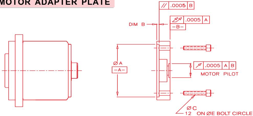
It is recommended that PSS/PSF gearheads be purchased with motor adapter kits supplied by Harmonic Drive Technologies. Contact our engineering department with the details of your motor interface.
