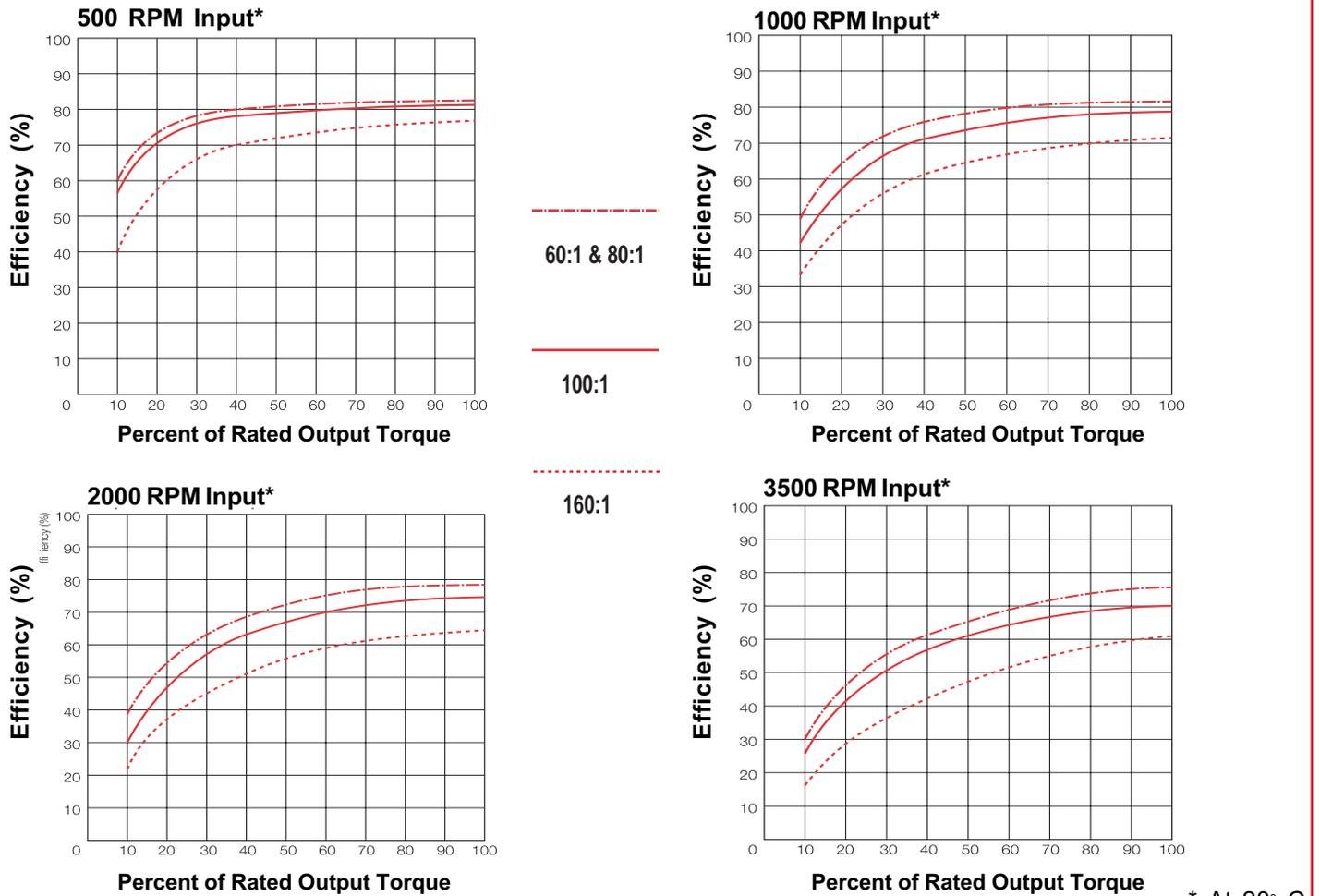
The efficiency of a Harmonic drive gearbox is dependent on speed, ratio, load and temperature. For convenience the above graphs show efficiency against percentage of rated output torque. In applications where the output torque is very low compared to the ratings or in extreme temperature consult our factory.
