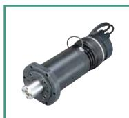
The precision lead screw provides positioning accuracy in the micron range  $\,$  with submicron repeatability. The actuator is capable of thrust forces up to 12,000 N.
