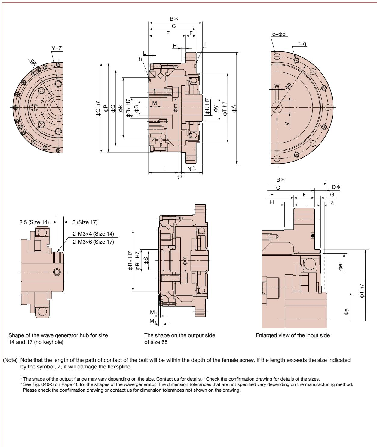
(Note) Note that the length of the path of contact of the bolt will be within the depth of the female screw. If the length exceeds the size indicated by the symbol, Z, it will damage the flex spline.
