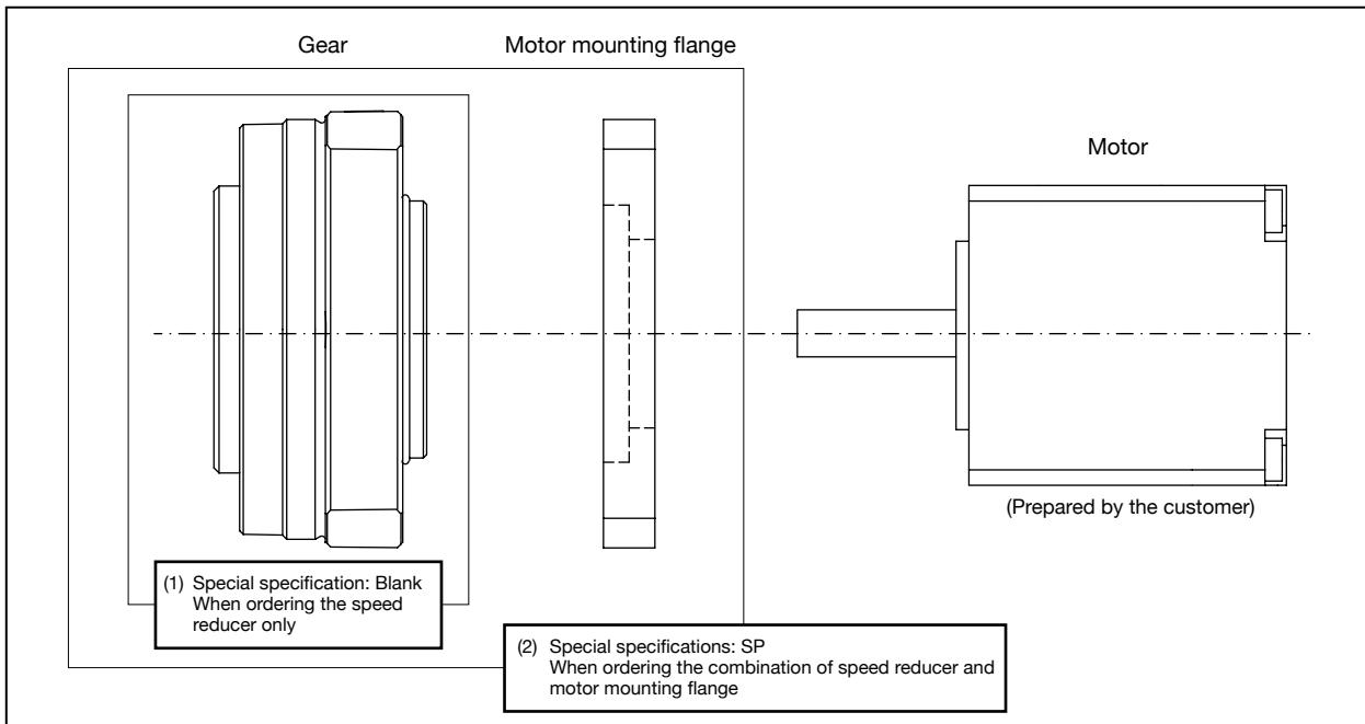
\* The motor mounting flange is designed and sold as an option. Please let us know the required dimension shown in Figure 168-1 on page 168 if you need the flange designed.
