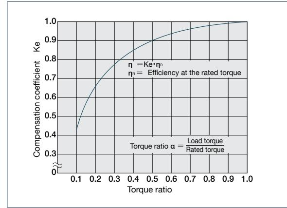
\* Efficiency compensation coefficient  $K_e=1$  holds when the load torque is greater than the rated torque.
