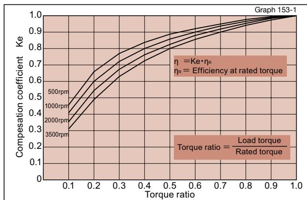
\*When load torque is larger than rated torque, efficiency compensation coefficient  $Ke = 1$ .
