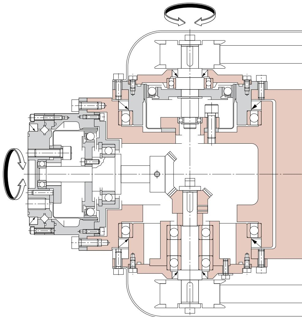
\*For this installation example, sealing is required to prevent grease leakage.
