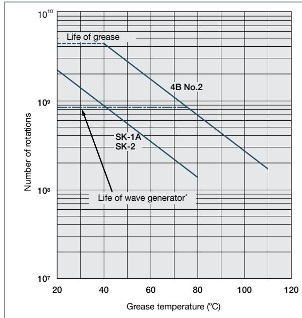
\* Life of wave generator is based on L10 life of the bearing.
