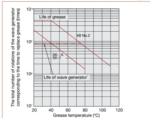
\* Life of wave generator is based on  $L_{10}$  life of the bearing.
