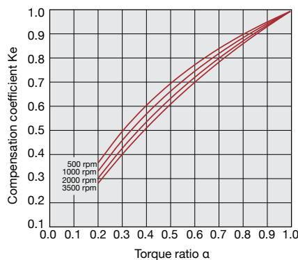
\* When the load torque is higher than the rated torque, efficiency compensation value  $K_e$  is 1.
