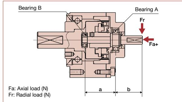
Relation between the radial load and the axial load
