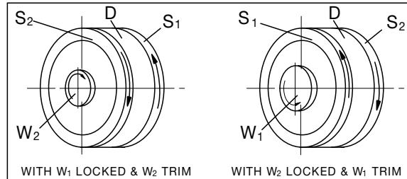
These examples show the displacement of the circular splines S1 and S2 relative to each other when the wave generator is rotated in the direction of the arrow. Actual rotational direction will depend on the direction of the main input drive.
