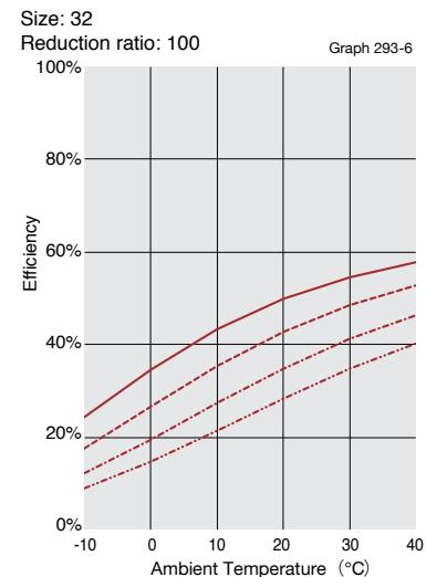
Input rotational speed ————— 500rpm ————— 1000rpm ————— 2000pm ————— 3500pm ————— 3500pm
