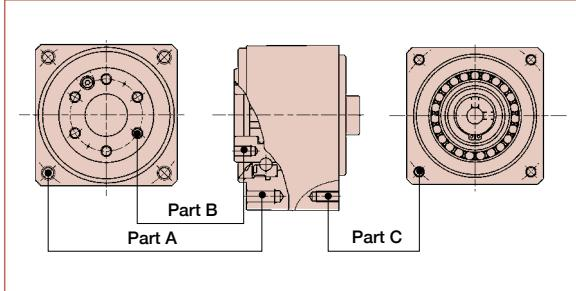
Avoid impact to the output flange during assembly. It may result in damage to the gearhead.
