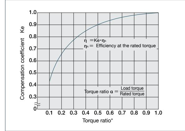
\* Efficiency compensation coefficient  $Ke=1$  holds when the load torque is greater than the rated torque.
