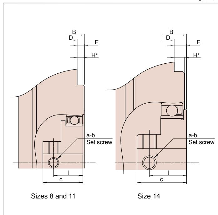
\* Dimension H is the mounting position in the shaft direction and tolerance of the three parts (wave generator, flex spline, circular spline). Strictly observe these dimensions as they affect the performance and strength.
