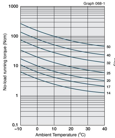
Input rotational speed: 1000rpm
