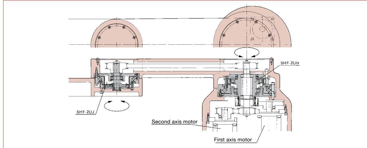
Typical example of a wrist joint arrangement in a gantry-type robot using SHF-2UH and SHF-2UJ gear units.
