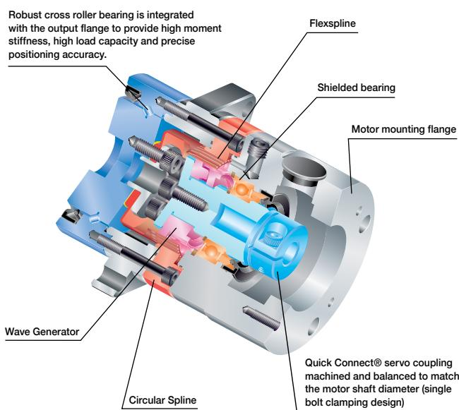
**CSF-GH and CSG-GH Quick Connect® gearheads** with zero backlash Harmonic Drive® gearing are available with high reduction ratios, 50:1 to 160:1. CSF-GH and CSG-GH utilize our proprietary S tooth profile and provide high precision positioning (repeatability  $\pm 4$  to  $\pm 10$  arc-sec). The greatest benefit of Harmonic Drive® gearing is the weight and space savings compared to other gearheads because it consists of only three basic parts.
