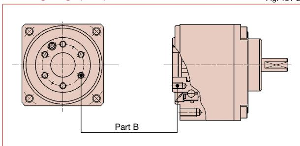
Do not allow the output shaft to receive a shock when you install a pulley and pinion. It can deteriorate the precision of the reducer and cause failure.
