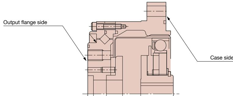
CSG series: Installation of output flange side and transmission torque
