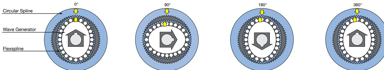
The Flexpline is slightly smaller in diameter than the Circular Spline and usually has two fewer teeth than the Circular Spline. The elliptical shape of the Wave Generator causes the teeth of the Flexpline to engage the Circular Spline at two opposite regions across the major axis of the ellipse.
