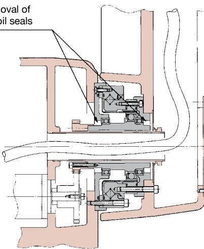
**Typical example of the use of SHF-2UH gear unit with rotary shaft seals removed.**
