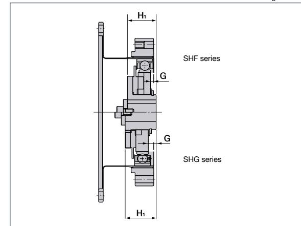
Comparison of Dimension of Wave Generator
