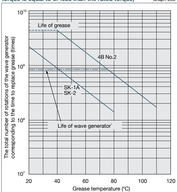
\* Life of wave generator is based on L10 life of the bearing.
