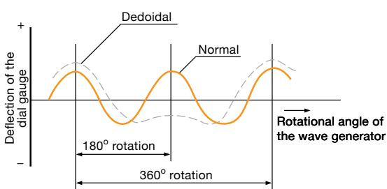
Measuring the deflection on the body of the flexspline
