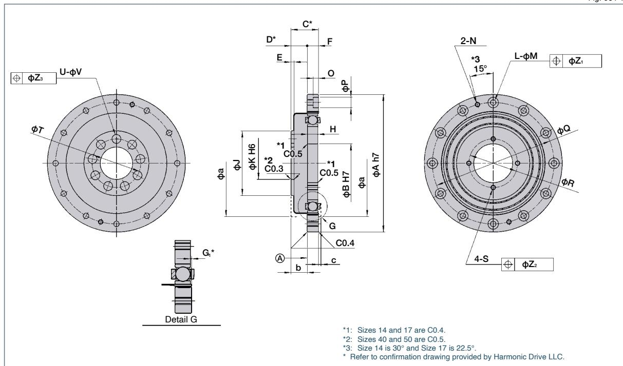
**■ Structure and shape of the wave generator**
