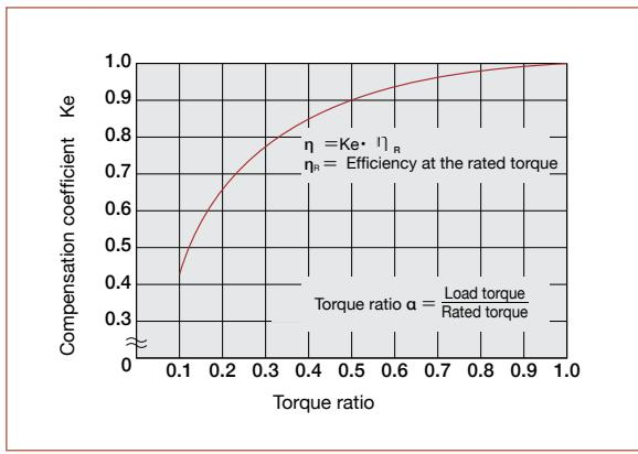
■ Efficiency at rated torque
