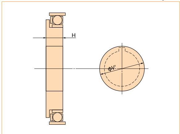
Hole diameter of the wave generator hub with Oldham coupling
