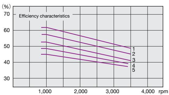
(Note) The efficiency decreases by about 10% for grease lubrication.
