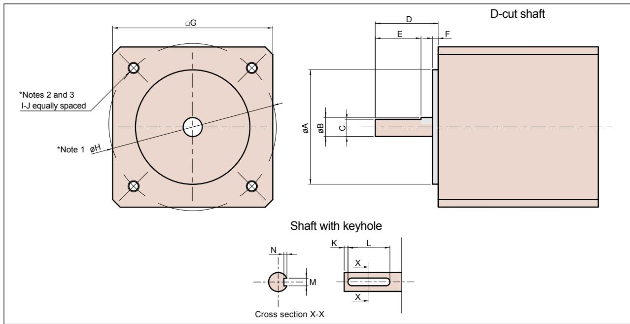
\* Note 1. H: Mounting hole pitch diameter or pitch angular dimension
