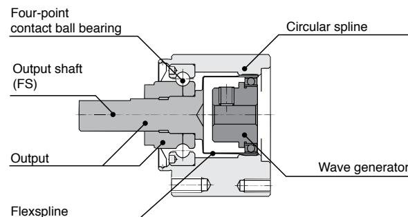
\* The rotational direction of the output shaft is opposite to that of the input shaft (wave generator) when the circular spline is fixed.
