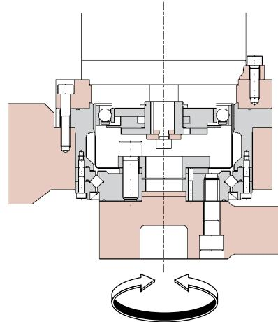
\* For usage as this installation example, sealing is required to prevent grease leakage.
