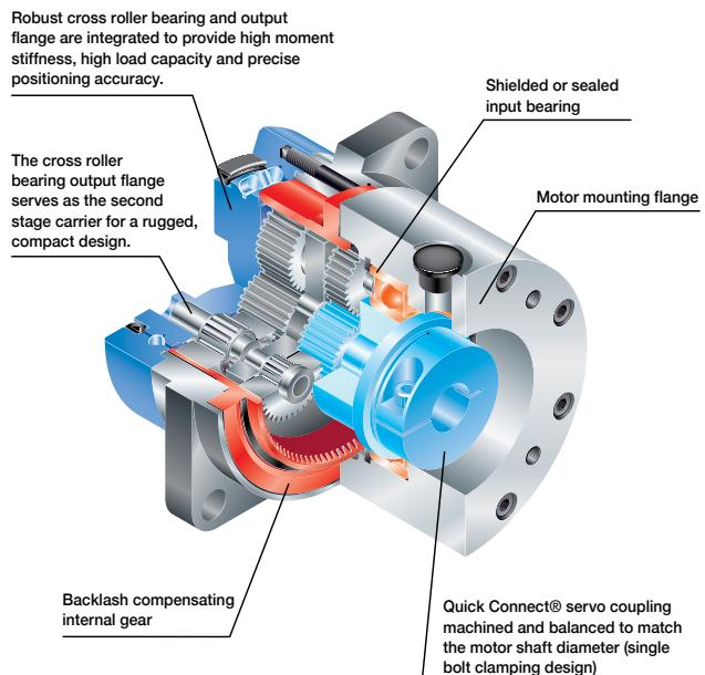
**HPG and HPGP Quick Connect® gearheads** offer high precision and low backlash (standard: < 3-arc-min, optional: <1 arc-min). Harmonic Planetary® HPG gearheads are now available with helical gearing and low reduction ratios. The new models, HPG-XX R, add low-speed ratios from 3:1 through 10:1 including all integer ratios in between. Innovative ring gear ensures consistent, low backlash for the life of the gearhead. Right Angle configuration also available.
