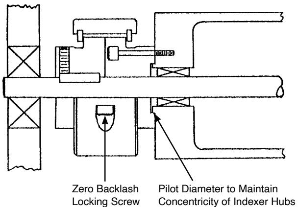
HDI Infini-Indexer phase adjuster used to manually phase a hollow roll to a solid through-shaft
