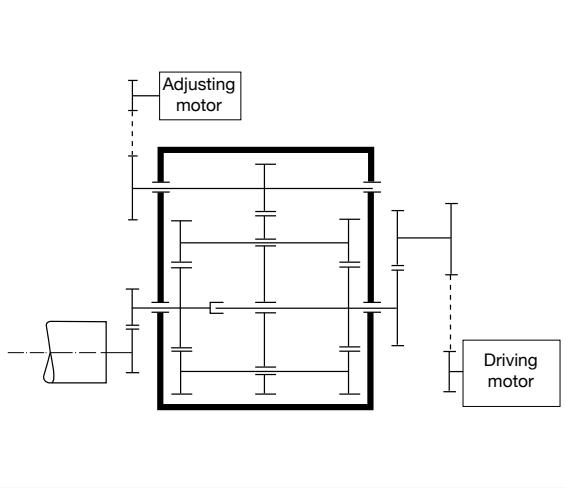
Using the Harmonic differential gear
