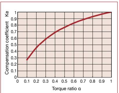
Note: When the load torque is greater than the rated torque the efficiency compensation coefficient  $K_e = 1$ .
