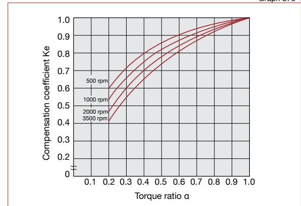
\* When the load torque is higher than the rated torque, efficiency compensation value  $K_e$  is 1.
