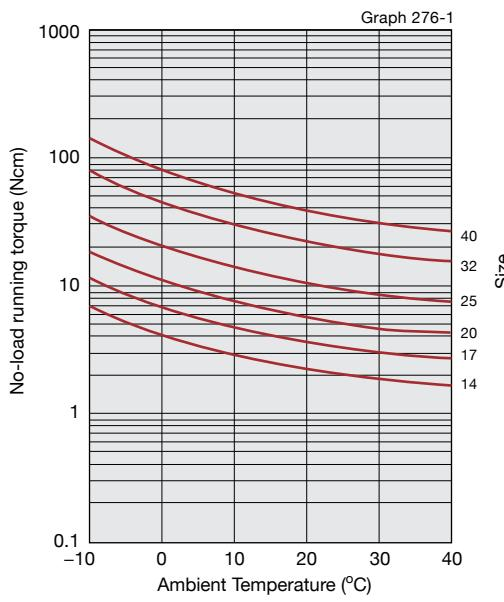
Input speed: 1000rpm
