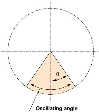
(Note) A small angle of oscillation (less than 5 degrees) may cause fretting corrosion to occur since lubrication may not circulate properly. Contact us if this happens.
