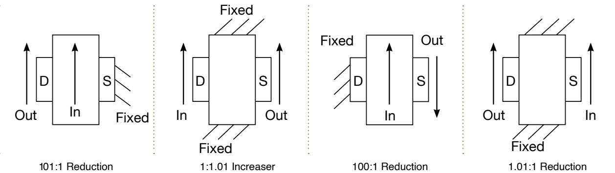
If any two elements are locked together, the indexer will not phase and the unit will rotate in a 1:1 mode.
