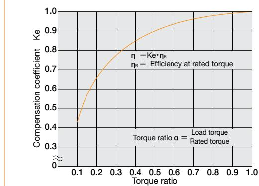
\* Efficiency compensation coefficient  $K_e=1$  when the load torque is greater than the rated torque.
