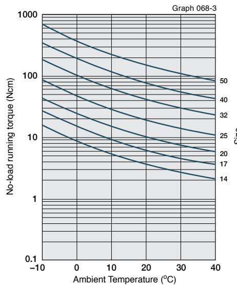
Input rotational speed: 3500rpm
