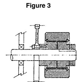
The Infinit-Indexer® phase adjuster can be installed in a machine system either as an in-line shaft coupling or a concentric shaft coupling.
