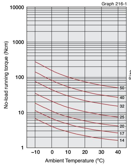
Input speed: 1000rpm
