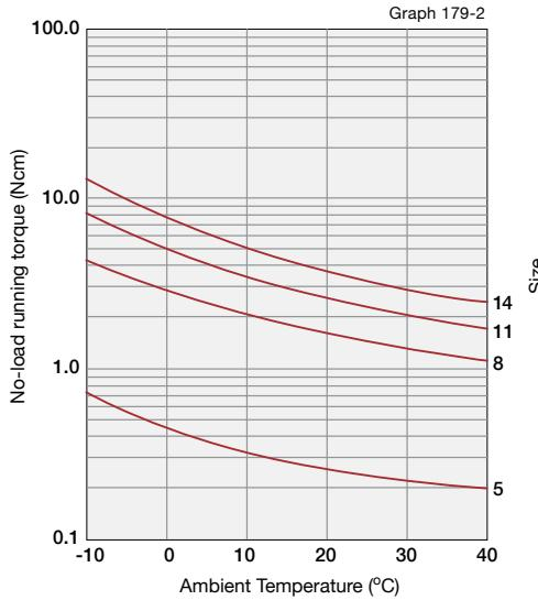
Input speed: 2000rpm
