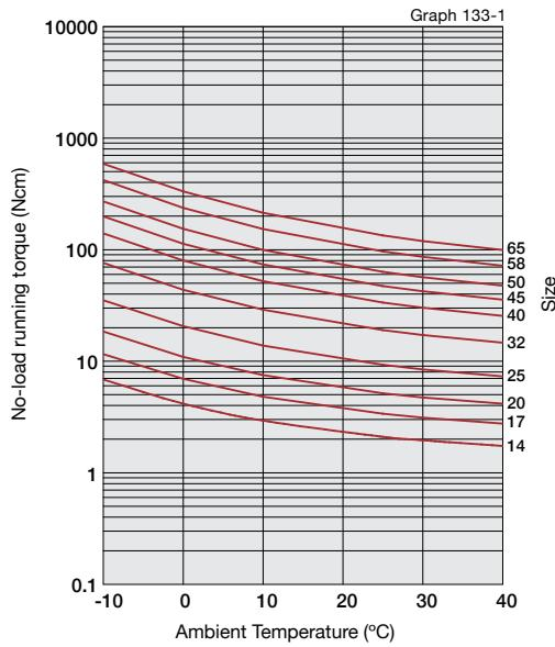
Input speed: 1000rpm
