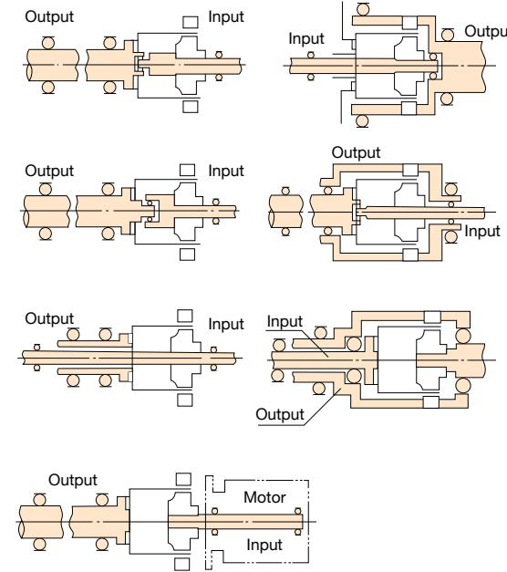
**Wave generator****■ Structure of the wave generator**
