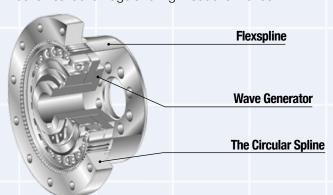
The **Wave Generator** is a thin ball bearing fitted onto an elliptical hub. This is generally mounted onto the input or motor shaft. As the hub is rotated, a pair of moving waves is produced on the outside of the non-rotating outer race of the bearing.
