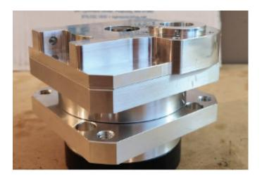
the call. Integrated with the output flange, the CRB provides a compact form factor and high resistance to impact due to the narrow, single row arrangement. The bearing is preloaded and rolling elements placed orthogonally to one another between the ground raceways.
