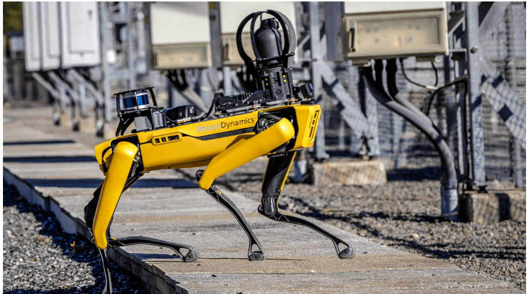
Spot is a general-purpose, four-legged mobile platform that weighs 60 lb. Image: Rightpoint
