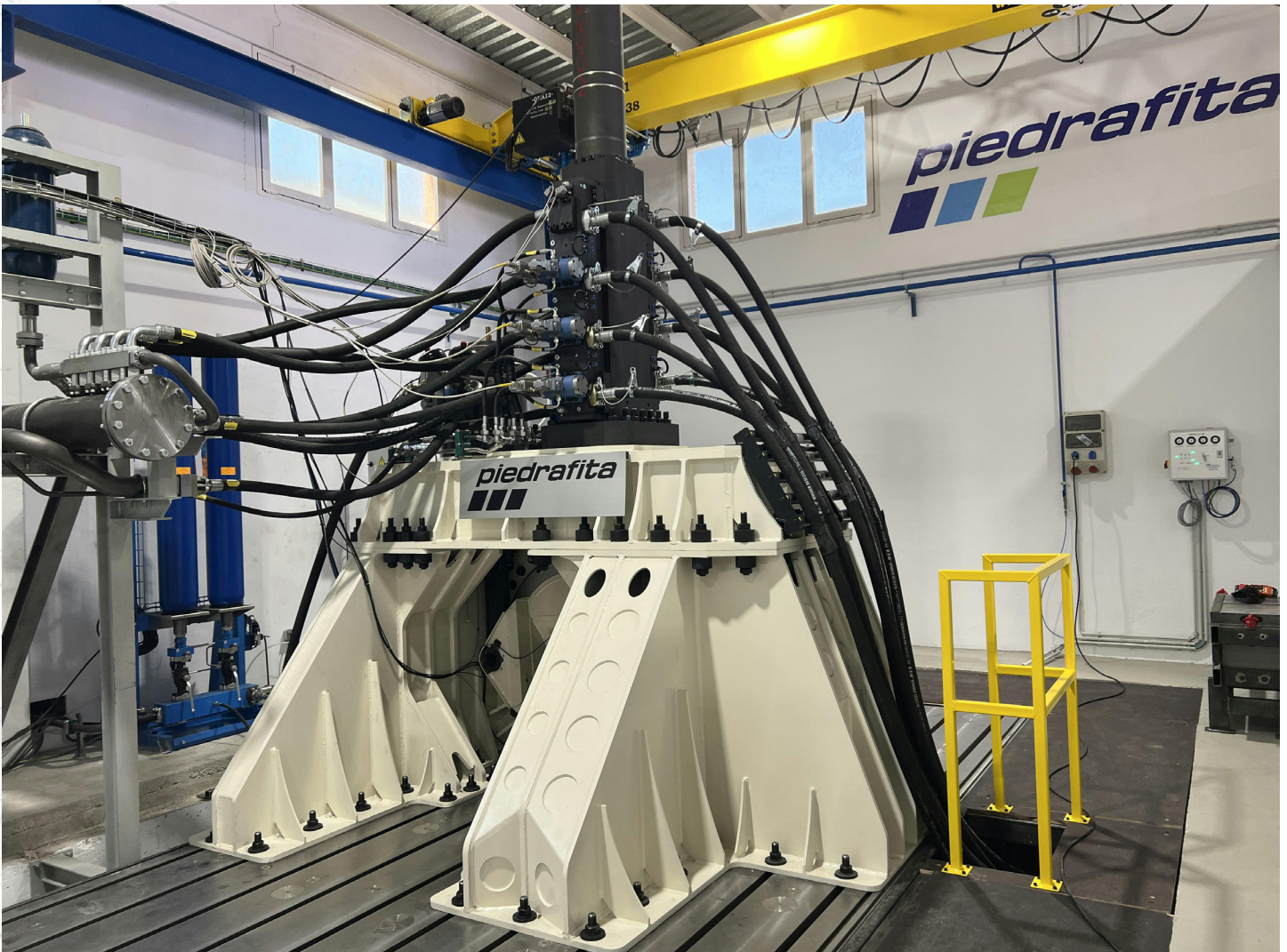
A custom-designed test bench developed by Moog and Piedrafita Systems simulates the movement of a hydraulic vehicle's tracks over uneven terrain. The system incorporates hydraulic actuators with digital servo valves, a test controller, power cabinet, digital pumps and an accumulator bench with piping. Moog
